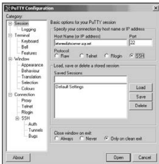
Figure 5.24 Establishing an SSH Connection to an Intermediate Computer on a Public IP Address
